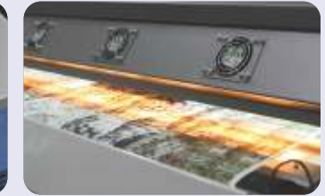
Under Fabric Heater & Tunnel Dryer
